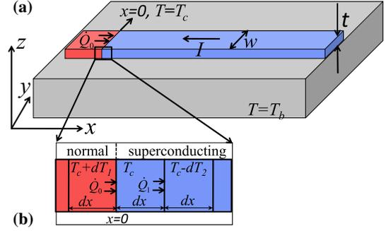
FIG. 2 (color online). (a) Schematic of the semi-infinite (in  $+x$  direction) lead of SC material on a substrate at  $T_b$  with an  $N$ - $S$  interface at  $x = 0$ . Panel (b) shows the region near the  $N$ - $S$  interface with three differential elements of length  $dx$  when the  $N$ - $S$  interface stabilizes near the heat source on the left.
