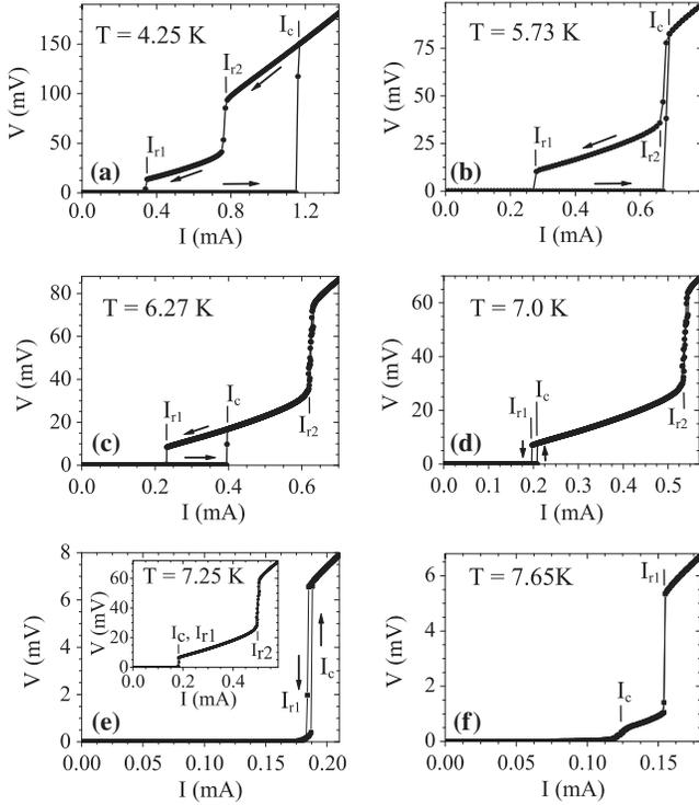
FIG. 3. (a)-(d) IVCs in the hysteretic regime for  $\mu S1$  at different temperatures. A large hysteresis is seen at 4.25 K with two retrapping currents,  $I_{r1}$  and  $I_{r2}$ .  $I_c$  crosses  $I_{r2}$  near 5.7 K and  $I_{r1}$  around 7.25 K as seen in (e). Panel (f) shows the IVC of  $\mu S1$  in the nonhysteretic regime above  $T_h = 7.25$  K. The inset of (e) gives a larger bias-current range plot to show the  $I_{r2}$  transition.
