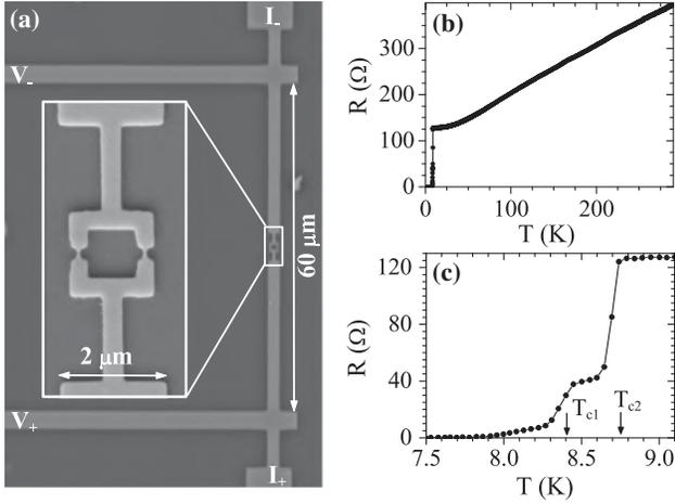
FIG. 1. (a) SEM image of the  $\mu$ -SQUID  $\mu S1$  with its current and voltage leads. The zoomed-in image shows the SQUID loop (with area  $1 \times 1 \mu\text{m}^2$ ) and the narrow leads. (b) Resistance versus temperature ( $R$ - $T$ ) plot. (c) Low-temperature portion of the  $R$ - $T$  plot for  $\mu S1$  at 0.01 mA current.
